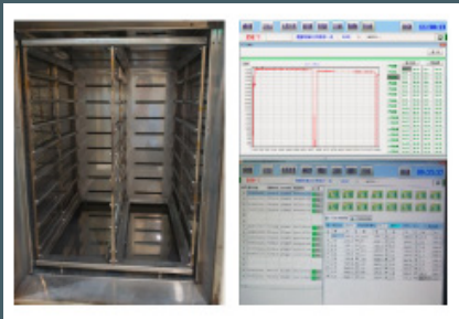
Figure 13: Burn-in process required to address early failures
